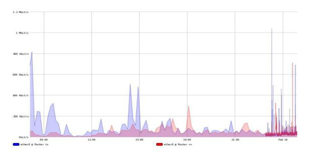
The graph show the data usage throught the network cable supplying the enterance and Food Vendors. This will also have data usage also from others roaming from one WiFi radio to another with cellphones etc.
