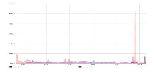
This graph shows how little data was transferred during the event. This is one of the reasons that the system worked so well due to the small packets of data to run the POS network.
